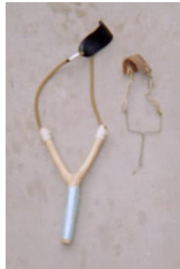
from broken planes. I cut the belt piece about 2 inches long and punch two small ¼ inch holes with sharpen hole punch I made from some old metal tubing.
